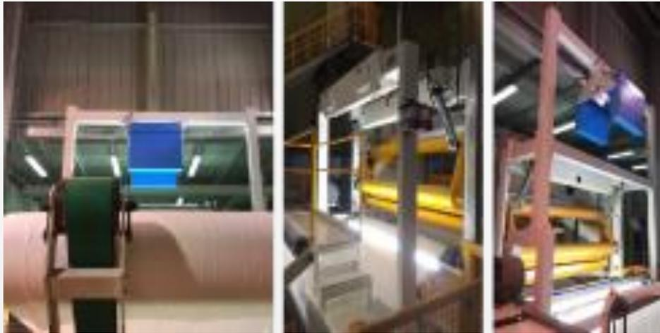
It can monitor the quality of coated paper, cardboard, special paper, sanitary paper, synthetic paper and other materials in real time, and carry out online detection of possible defects.
