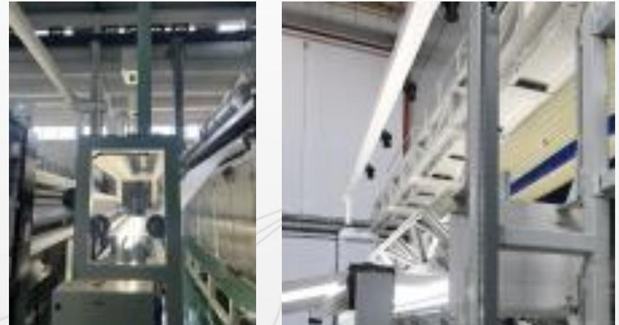
It can monitor the quality of various non-woven materials such as spun-bonded non-woven cloth, water-borne non-woven cloth, needle-spun non-woven fabric, hot-rolled non-woven cloth, and detect the possible defects online.
